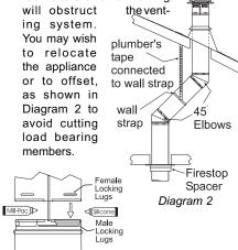
Note: Apply sealant "Mill-Pac" to inner pipe and high temperature silicone sealant to outer pipe on every twist-lock joint.
